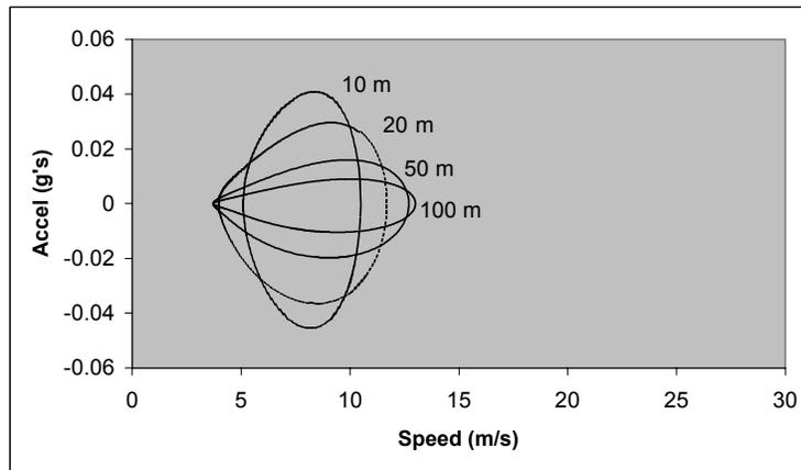
**Figure 5-4. Effect of Increased Hill Size on an Unfaired Vehicle**
