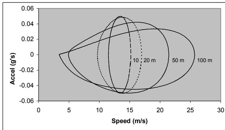
**Figure 5-5. Effect of Hill Height on Faired Vehicle Performance**
