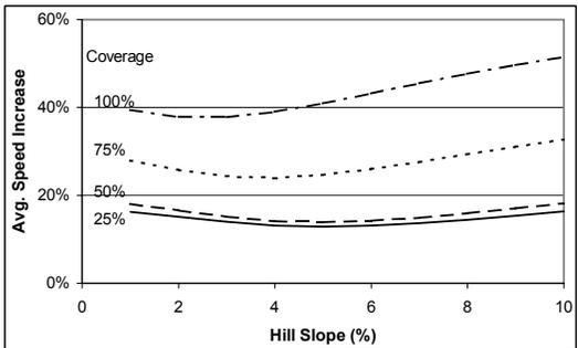
**Figure 5-8. Speed Increase due to Fairing Coverage – 50 m Hill**
