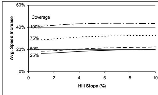
**Figure 5-6. Speed Increase due to Fairing Coverage – 10 m Hill**
