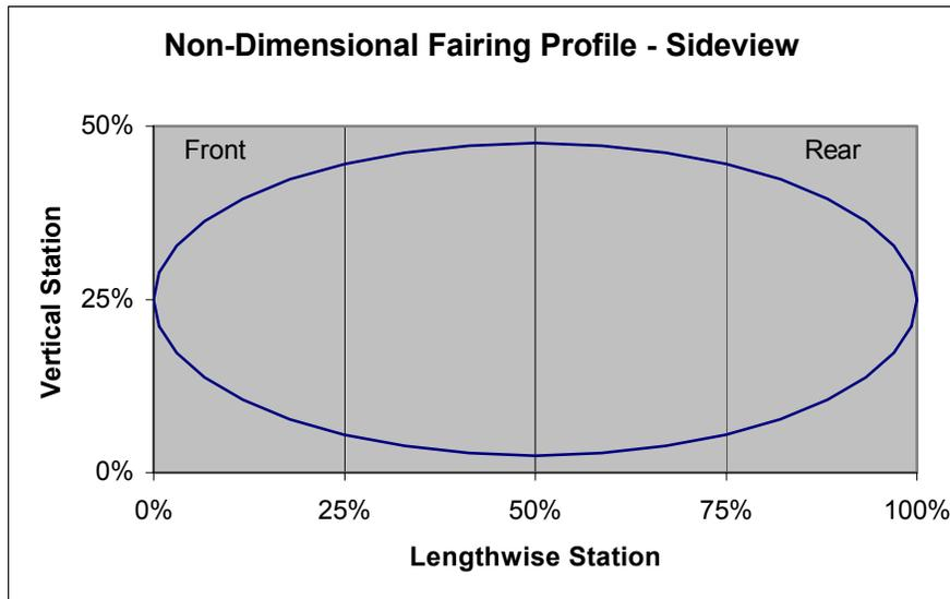
**Figure 3-4 Non-Dimensional Profile for Ellipsoidal Fairing**
