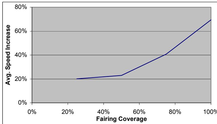
**Figure 3-6. Speed Increase with Fairing Coverage**
