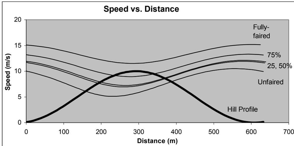
**Figure 5-1. Increasing Fairing Coverage on a Constant-sized Hill**
