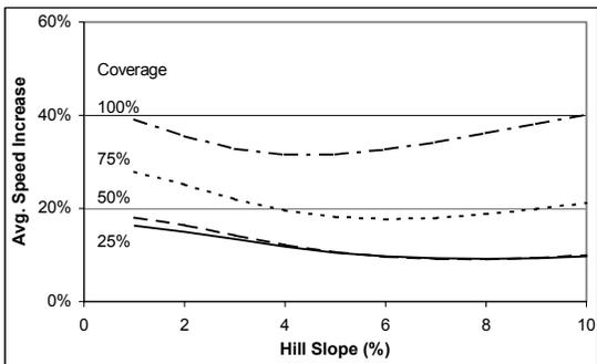
**Figure 5-9. Speed Increase due to Fairing Coverage – 100 m Hill**
