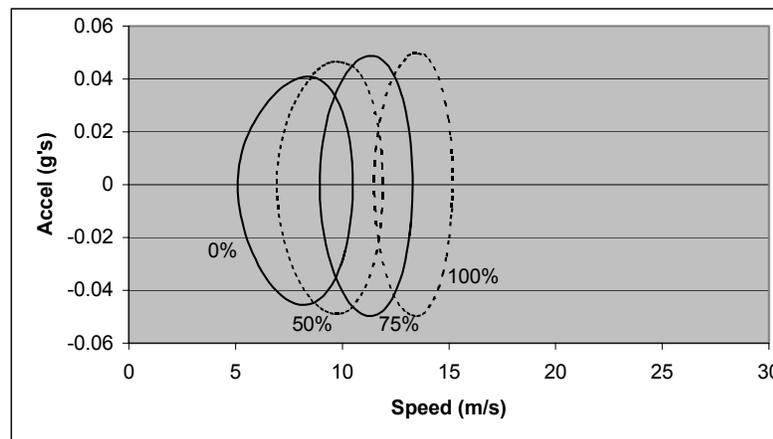
**Figure 5-3. Phase Plot Showing Effect of Fairing Coverage (10m Hill – 5% Grade)**
