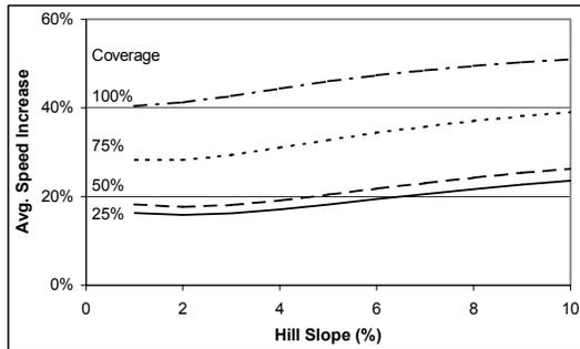
**Figure 5-7. Speed Increase due to Fairing Coverage – 20 m Hill**
